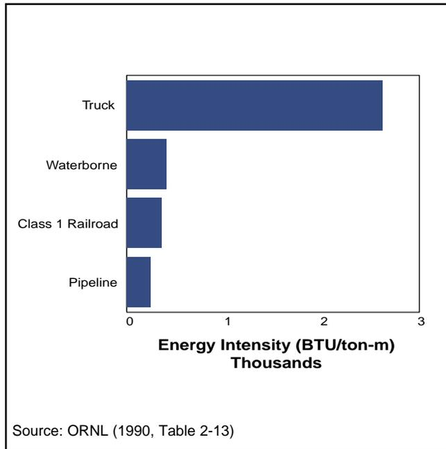
Figure 4.9-1. Energy intensity for freight shipments, 1997. Crude oil and product pipelines are relatively efficient.
