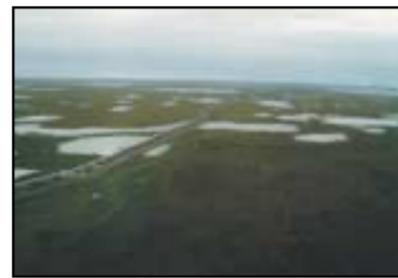
**North Slope:** Elevated pipeline over ice-rich permafrost on the Arctic Coastal Plain near Prudhoe Bay (MP 4)
