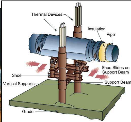
Vertical support members consist of crossbeams installed between vertical supports placed in the ground. The above-ground pipe is insulated, jacketed with galvanized steel, and mounted on a Teflon-coated shoe that can slide back and forth on the VSM crossbeams.
