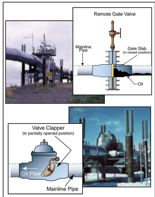
Figure 2.1-3. TAPS gate valve (top) and check valve (bottom). (Alyeska photos)
