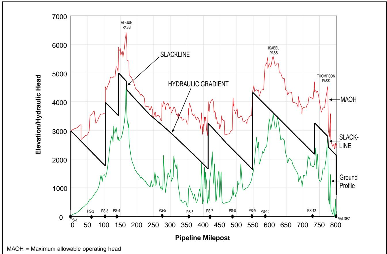
Figure 2.1-7. Hydraulic gradient graph for operating condition of 1.1 million bbl/day with Pump Stations 1, 3, 4, 7, 9, and 12 operating; Pump Stations 2, 6, 8, and 10 on standby; and Pump Station 5 as a pressure relief station.
