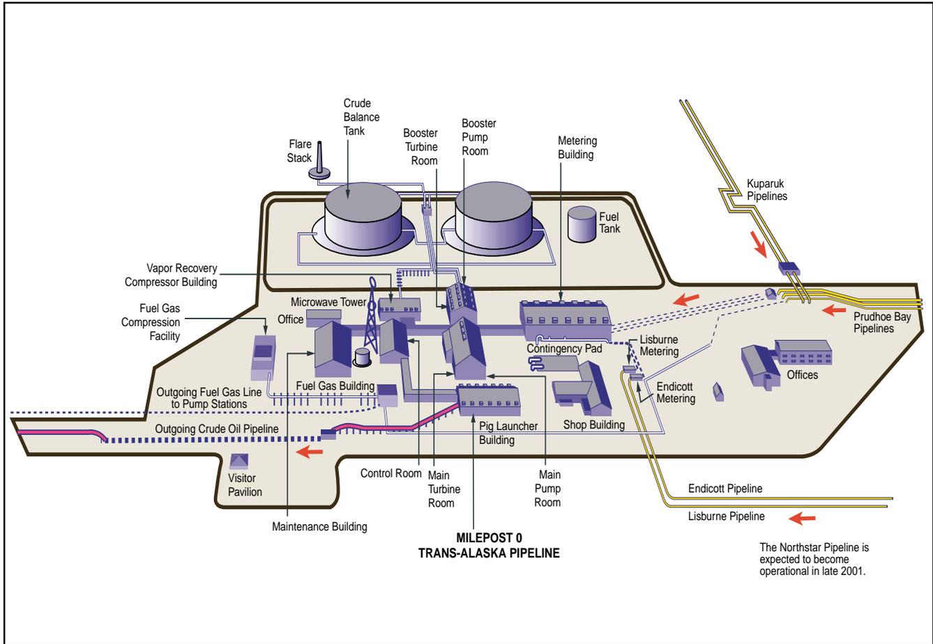
Figure 2.1-4. Pump Station 1 at TAPS Milepost 0.
