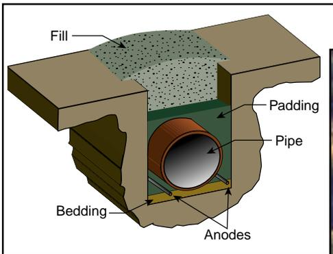
Pipeline buried in the standard method lies on a layer of bedding material (well-drained sandy gravel without sharp rocks) covered with prepared gravel padding and soil fill material. The photo at right shows a transition between elevated and buried pipe.
